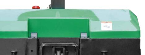
The components and connectors of the electrical system are mostly designed with high protection levels and placed inside the covering parts. The waterproof level reaches IPX4, which can meet the needs of outdoor operations.
