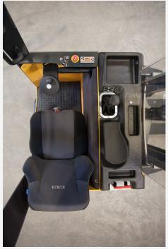
Adjustments The steering unit is fully adjustable. Further away, closer to the driver, changing angles etc. Stepless height controlled floor with angle adjustment.
