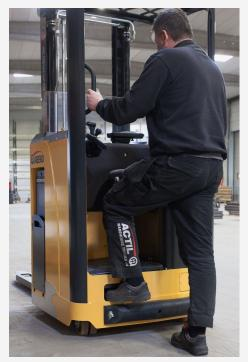
**Step-in** On SW 1350/1600 the step-in is only 230mm which helps the entry and exits from the forklift.
